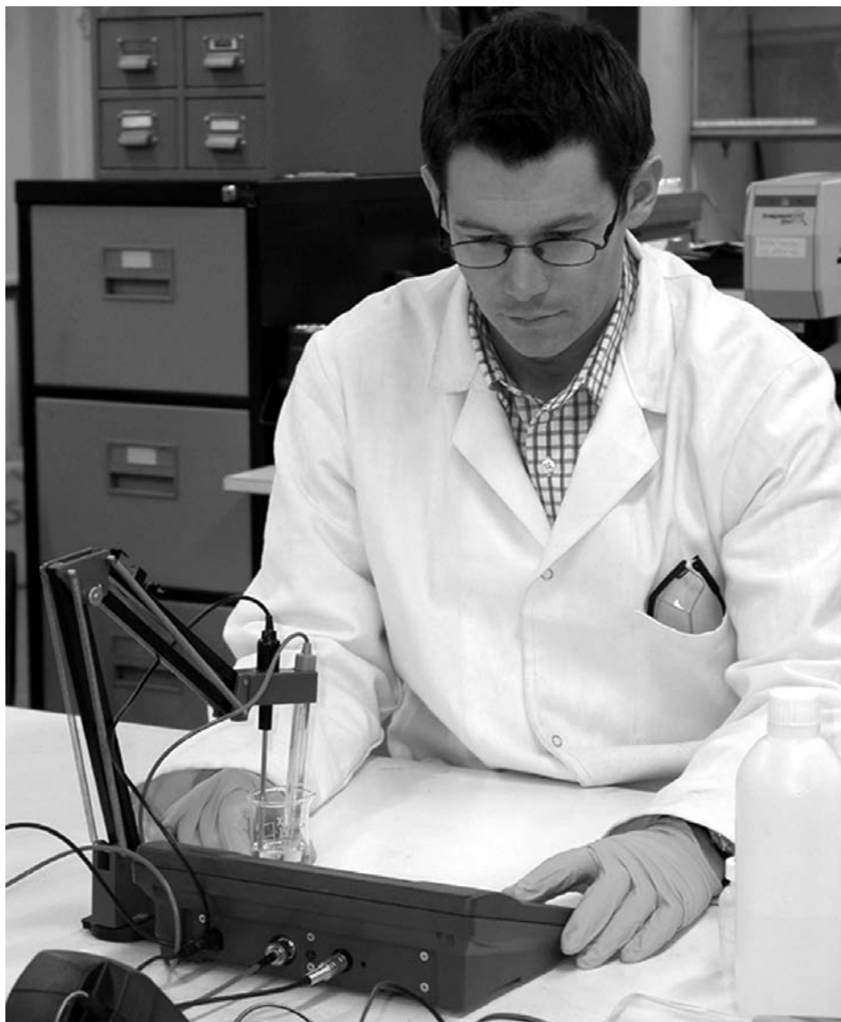
Recording the pH of an aqueous extract from an adhesive film
