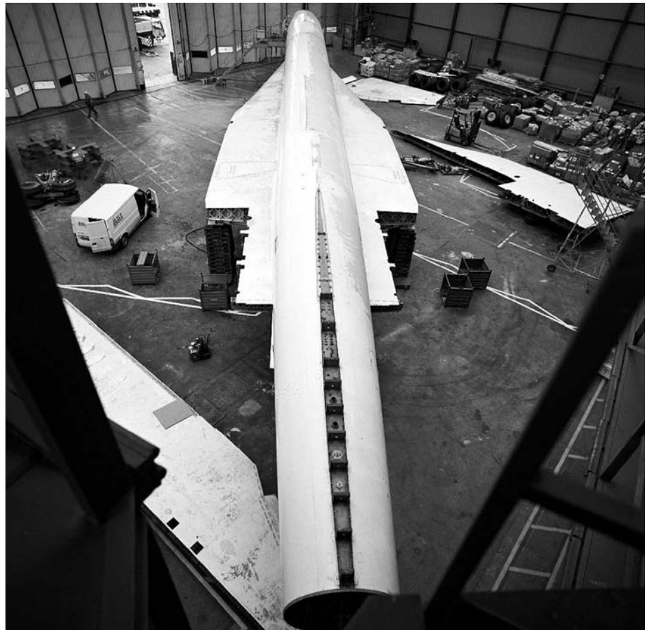
Right, the aircraft had to be reduced in size to be transported by road out of Heathrow. Below, Concorde's slow journey to the barge at Isleworth
