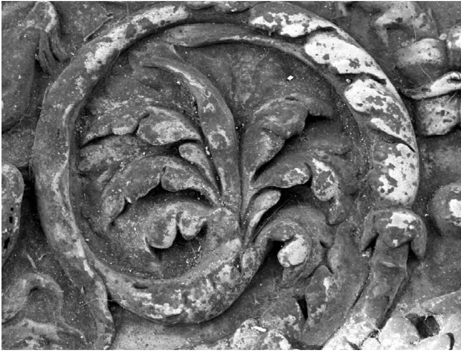
Example of some typical corrosion products found on an outdoor bronze feature in an urban environment, mainly in the form of copper sulphates and
